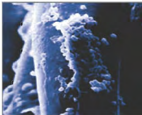
Untreated polymer shows growth of bacteria on polymer surface
